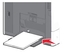
**6** From the printer control panel, set the Paper Size and Paper Type for the multipurpose feeder (MP Feeder Size and MP Feeder Type) based on the paper or specialty media loaded.
